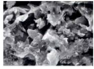
Macrolite particles are remarkably uniform and have greatly enhanced surface features that significantly enhance filtration contact area
